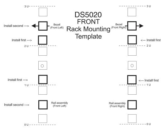
Figure 13. Front rack mounting template
